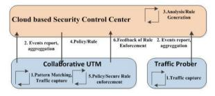
Figure 2. The work principle of CNSMS with Cloud based Security Center.
